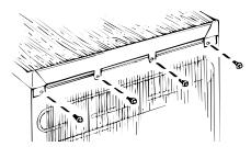
Take out four screws at the top rear of the cabinet, lift the top slightly at the rear and push it forward to remove it.
